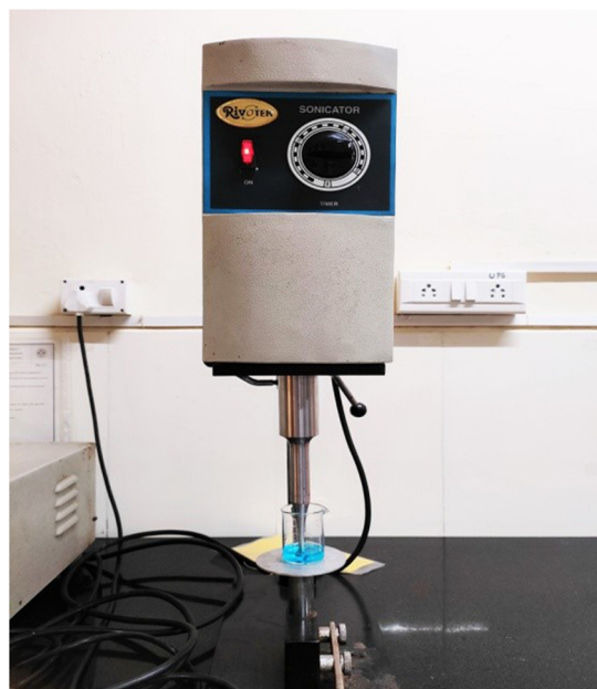
Figure 2: The green UAE technique for sample extraction.
