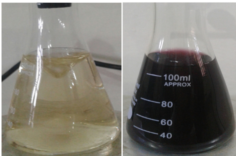
Figure 3: Change in color of the prepared PP-AuNPs.
