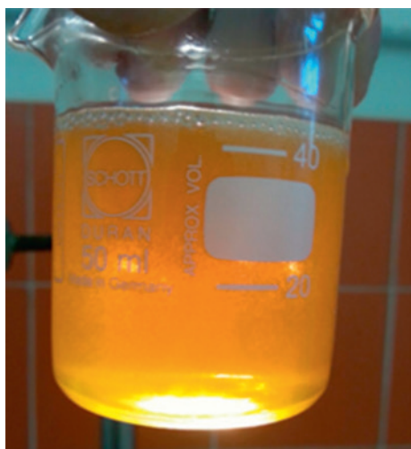
Figure 2: Dispersion of fine air bubbles in oil after treatment with the rotor-stator generator of HC.
