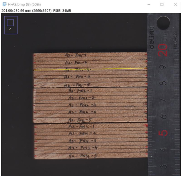
Figure 2: Diagram of strain measurement of the specimen by ImageJ.
