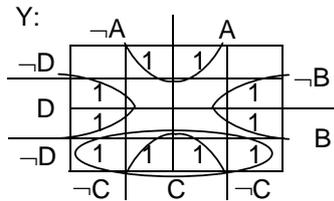
$$Y = (\overline{D} \wedge C) \vee (D \wedge \overline{C}) \vee (\overline{D} \wedge B)$$
