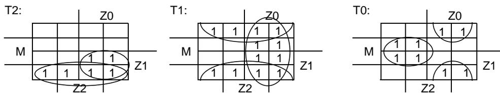
$$T2 = (Z1 \wedge Z0) \vee (\overline{M} \wedge Z1)$$
