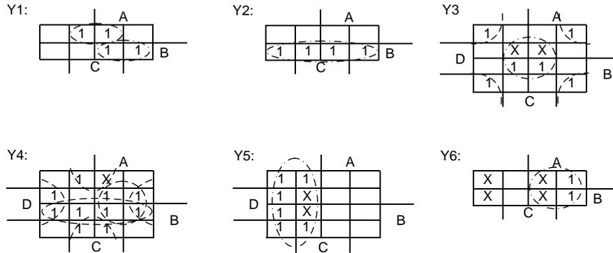
$$Y1 = (\overline{B} \wedge C) \vee (A \wedge B); \quad Y2 = B; \quad Y3 = (\overline{D} \wedge \overline{C}) \vee (D \wedge C) = D \leftrightarrow C$$
