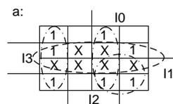
$$g = I3 \vee (I2 \wedge \overline{I1}) \vee (I1 \wedge \overline{I0}) \vee (\overline{I2} \wedge I1)$$
