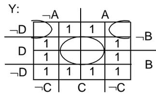
$$\overline{Y} = (D \wedge C) \vee (\overline{D} \wedge \overline{C} \wedge \overline{B}) \Rightarrow Y = (\overline{D} \vee \overline{C}) \wedge (D \vee C \vee B)$$
