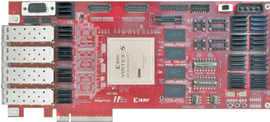
FIGURE e6.9.1 The NetFPGA 10-Gigabit Ethernet card (see http://netfpga.org/ ), which connects up to four 10-Gigabit/sec Ethernet links. It is an FPGA-based open platform for network research and classroom experimentation. The DMA engine and the four “MAC chips” in Figure e6.9.2 are just portions of the Xilinx Virtex FPGA in the middle of the board. The four PHY chips in Figure e6.9.2 are the four black squares just to the right of the four white rectangles on the left edge of the board, which is where the Ethernet cables are plugged in.
