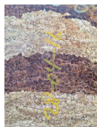
• Section of a Strand Woven Bamboo (SWB) product.
