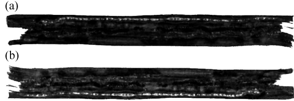
Fig. 1. Thin white track appearing near (a) the upper and (b) the lower boundary of the sample, after the spark has run from the cathode (on the left) to the anode (on the right). The length of the samples of 5 cm gives the scale of the photo.
