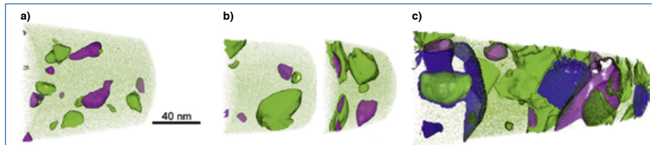
Fig. 16: APT reconstruction of an equiatomic CrMnFeCoNi high entropy alloy sample, aged at 450°C over different periods of time: a) 5 min, b) 1 h and c) 15 h. The iso-concentration surfaces represent the following regions: > 70 at.% Ni + Mn (green), > 50 at.% Cr (purple) and > 35 at.% Co (blue). Prior to thermal aging, APT could not detect any decomposition, meaning that the alloying atoms involved were homogeneously distributed in the solid solution [77].
