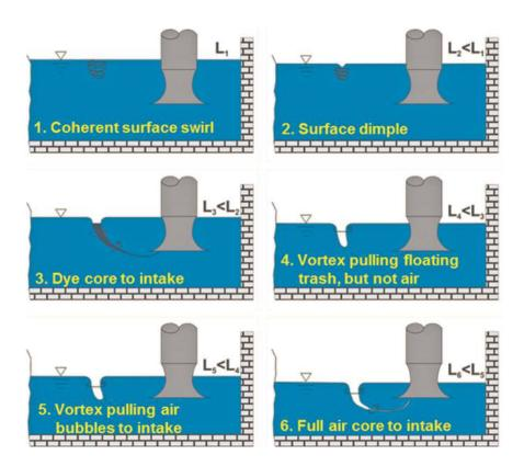
Fig. 1. Phases of surface vortex building by decreasing submergence
