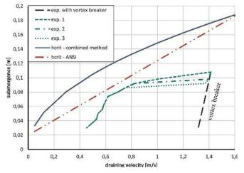
Fig. 8. Results of the draining tests and the critical submergence from combined method and ANSI correlation
