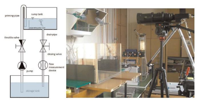
Fig. 3. Setup of the experiment and the PIV camera [8]
