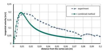
Fig. 7. Calculated and measured tangential velocity distribution (0.44 m/s)
