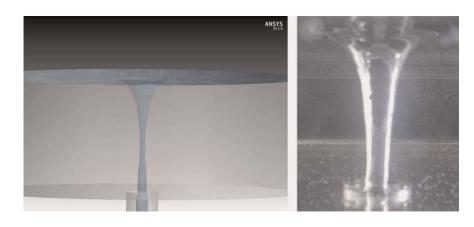
Fig. 5. Calculated (left) and the during the experiment observed surface vortex (right) [8]
