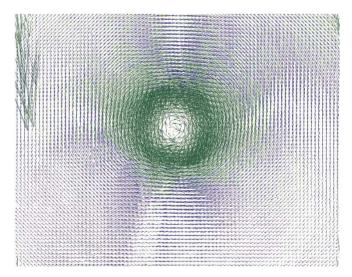
Fig. 4. The rotation symmetrical flow field measured in experiment with PIV [8]
