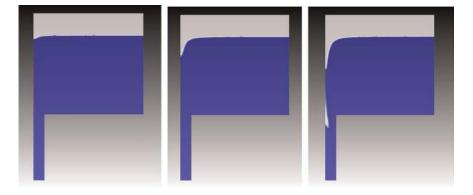
Fig. 6. Phase boundary at different intake velocities, blue: water and white: air (0.1, 0.25, 0.44 m/s)
