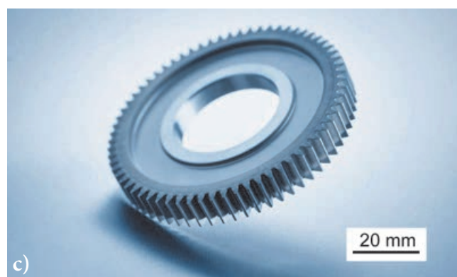
Fig. 9. Carburizing of surface densified PM gears, a) section of gas carburized gear, b) section of low pressure carburized gear, c) PM gear, low pressure carburized
