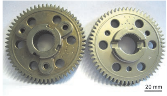
Fig. 11. PM steel gears oil quenched and washed (left) and high pressure gas quenched (right)
