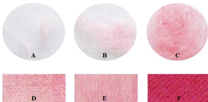
Figure 3. Surface images of wool fibers (A,B,C) and woven fabric (D,E,F) stained with Sirius red (A, D) before enzyme treatment, (B, E) after tyrosinase treatment, (C, F) after tyrosinase treatment and simultaneous coating with collagen.
