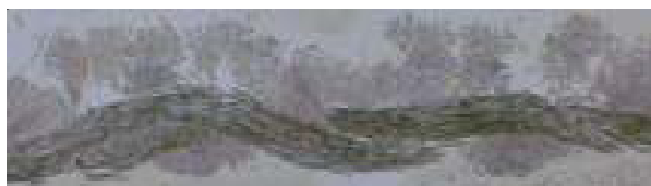
Figure 9. Transverse cross section-in satin fabric with warp sett=16 ends/100mm.
