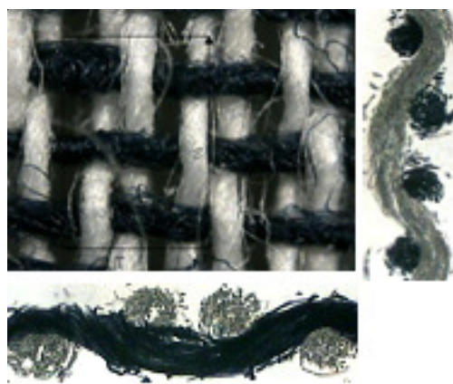
Figure 1. Depiction of real woven fabric and its longitudinal and transverse cross-section.
