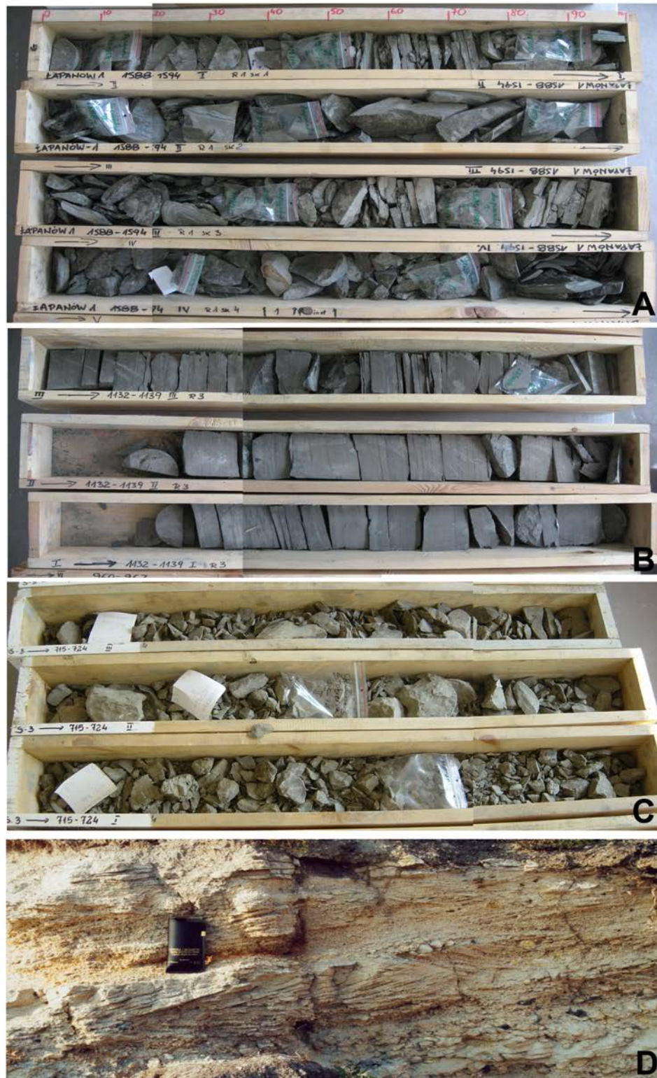
Figure 9. Typical lithofacies of the Middle Miocene of the PCF (outer foredeep). A - dark-grey, laminated marly siltstones and marlstones, upper part of the Skawina Fm. (Badenian), Łapanów 1 borehole, core interval 1,588-1,594 m; B - dark-grey, laminated claystones and mudstones of the Chodenice beds (Badenian/Sarmatian) with sporadic intercalations of grey, very thin-bedded (up to 0.5 cm), very fine-grained sandstones. Sandstones sometimes display ripple-cross lamination, Łukanowice 1 borehole, core interval 1,132-1,139 m; C - dark-grey laminated silty heteroliths, with horizons of ripple-cross laminated very fine-grained sandstones and siltstones. Upper part of the Machów Fm. (Sarmatian), Stobierna-3 borehole, core interval 715-724 m; D - Early Sarmatian littoral cross-laminated lamy sands, marginal part of PCF, NE of Pińczów [4].
