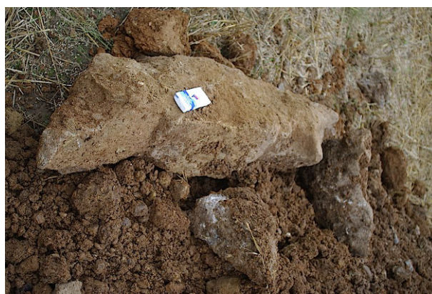
Figure 9. Nagelfluh blocks weighing up to several 100 kg and having been lifted up to 1 m from the perforation in Thunderhole #2. Length of tissue bag, 11 cm.
