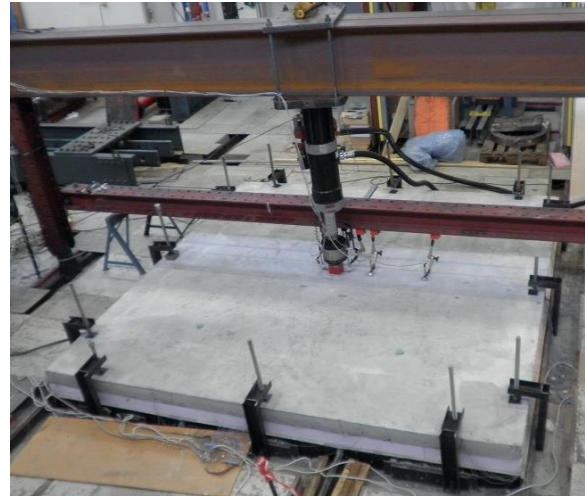
Figure 3. Ground slab and test set-up [15].
