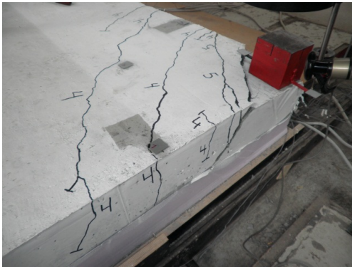
Figure 12. Crack patterns at failure for corner loading [15], (a) Corner load 1, (b) Corner load 2.
