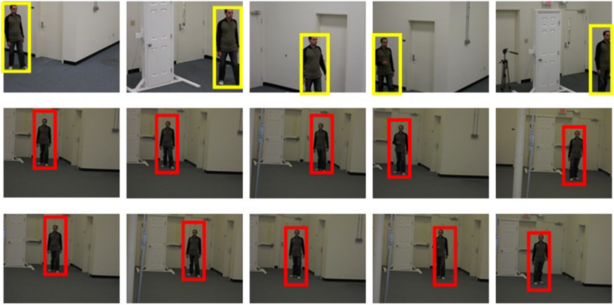
Figure 10. Performance of our proposed and reference methods for a real-time multiple PTZ cameras system. The first row shows five different locations in images of the j^{th} PTZ camera, the second row shows their respective pixel locations and sizes, derived by our approach, in images of the h^{th} PTZ camera, and the third row shows respective pixel locations and sizes, derived by Chen and Wang's approach, in images of the h^{th} PTZ camera. In this experiment, the single object is far away (18 meters) from the h^{th} PTZ camera (The tilt angle of the h^{th} PTZ camera is about 17^\circ )
