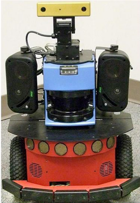
Figure 1. The robotic platform with the LIDAR system (blue and black section) and mounted camera (top).
