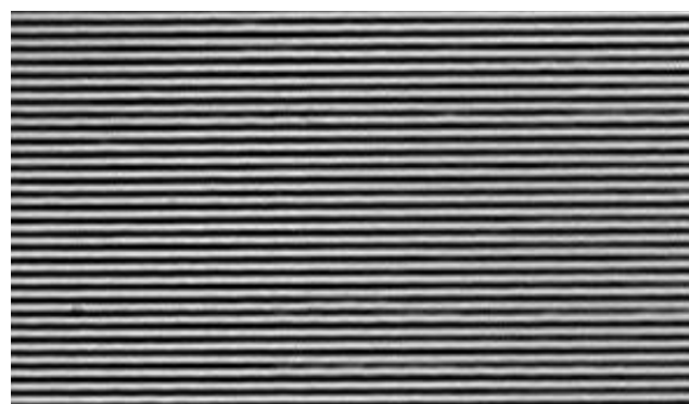
Fig. 5. Microscope image of grating coupler of the groove density \chi = 1000 g/mm.
