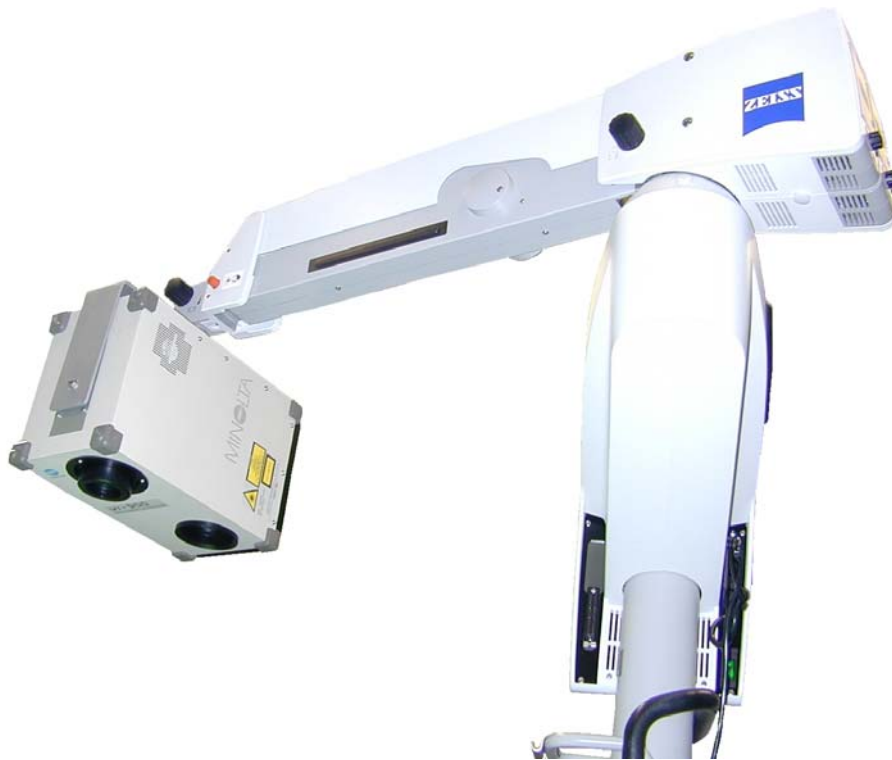
Fig. 1 Laser surface scanner mounted on an adjustable stand.
