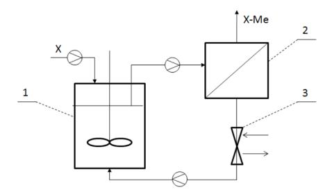
Figure 1. Flowchart of the production of mineral feeds additives based on algal biomass. (1): Reactor/biosorber (here the biosorption process takes place), (2): Filter (here the separation of the biomass from permeate takes place), (3): Valve [13].
