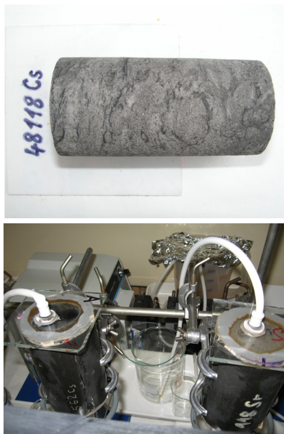
Figure 1. Core sample of the fucoidic sand and a part of the experimental setup
