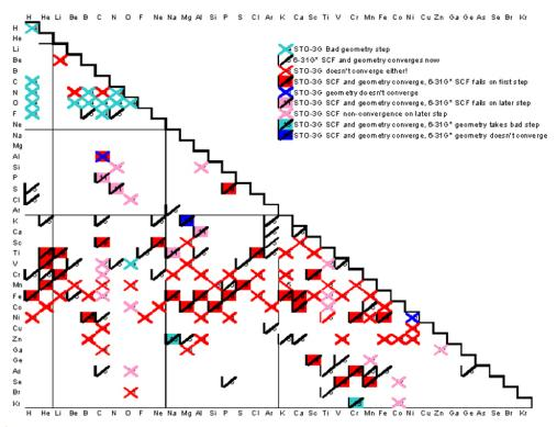
Figure 3. Results of running HF/STO-3G optimization, followed by HF/6-31G\* optimization calculations on the Set 1-4 molecules starting with the STO-3G geometry (but not the wavefunction). A black checkmark indicates the HF/STO-3G geometry calculation was successful. A red X indicates the HF/STO-3G SCF calculation failed to converge on first step, a pink X indicates that the HF/STO-3G calculation failed at a later step, a blue X indicates that the HF/STO-3G geometry failed to converge.
