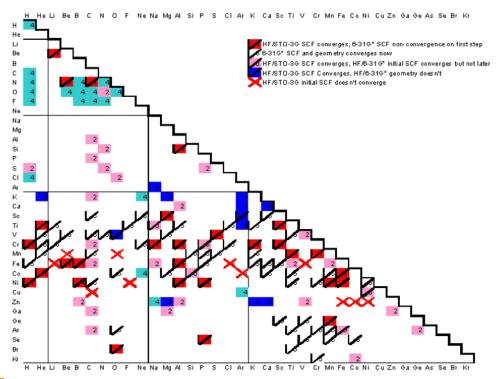
Figure 2. Results of running HF/6-31G\* optimization calculations on the Set 1 molecules. A black checkmark indicates the HF/STO-3G SCF calculation was successful. A red X indicates the HF/STO-3G calculation failed to converge.
