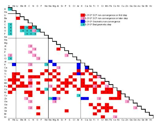
Figure 1. Results of running HF/6-31G\* optimization calculations on the test set. The position in the figure identifies the particular diatomic. White indicates normal completion. Red values indicate that the SCF failed to converge on the first step. Pink values indicate that the SCF failed to converge at some later geometry step. Blue values indicate that the geometry did not converge. Green values indicate that the geometry took a bad step which resulted in an optimization error.
