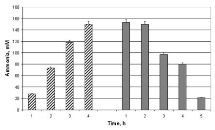
Figure 6. Quantity of ammonia released, corresponding to the quantity of degraded substrate-mixture of tolunitriles in the bioreactor; Sate of the process; second step
