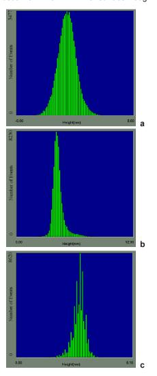
Figure 3. AFM and roughness analysis of synthesized hybrid materials containing TEOS and different percent k-carrageenan (a) 5 wt%; (b) 10 wt% and (c) 20 wt%
