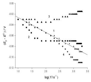
Figure 6. Dependence of the net peak potential on the logarithm of frequency. K = 0.01 cm,  $k_{\text{ads}} / \text{ cm s}^{-1} > 10^4 (1)$ , = 1.6 (2), 0.03 (3) and 30 (4). All other parameters are as in Fig. 1.
