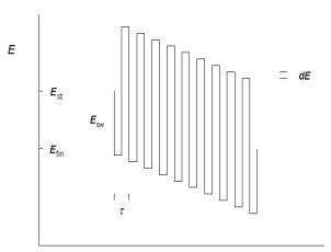
**Scheme 1.** Excitation signal of the square-wave voltammetry.  $E_{_{SW}}$  pulse height, dE potential increment,  $\tau$  staircase period,  $E_{_{SI}}$  starting potential,  $E_{_{fin}}$  final potential.
