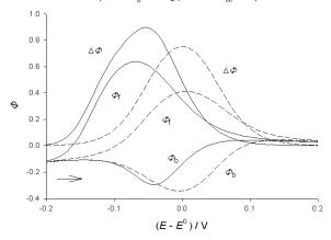
Figure 1. Square-wave voltammograms of electrode reaction (1) unaffected by the reactant adsorption (K'= 0) (a broken line), and influenced by the fast, equilibrated adsorption of reactant (K' = 33.33 and k' <sub>ads</sub> > 10 $^5$ ) (a full line).  $E_{sr} = -0.3 \text{ V}$  vs E', dE = 5 mV and  $E_{sw} = 50 \text{ mV}$ . A net response ( $\Delta \Phi$ ) and its forward ( $\Phi_p$ ) and backward ( $\Phi_p$ ) components are hown.
