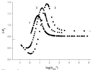
Figure 2. Dependence of dimensionless net peak current of square-wave voltammograms of electrode reaction (1) on the logarithm of dimensionless rate constant of the reactant adsorption. *K*\*= 3.33 (1, ♦), 10 (2, ▲) and 33.33 (3, ●). All other parameters are as in Fig. 1.
