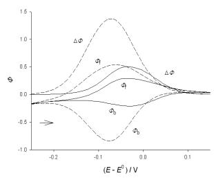
**Figure 3.** Square-wave voltammograms of electrode reaction (1) influenced by kinetically controlled adsorption of reactant.  $K^* = 33.33$  and  $k^*_{ads} = 1$  (a full line) and 53.33 (a broken line). All other parameters are as in Fig. 1.
