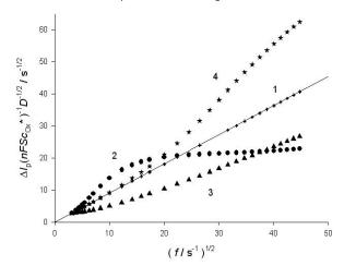
**Figure 4.** Dependence of normalized net peak current on the square-root of frequency. K = 0.01 cm,  $k_{\rm ads}$  / cm s $^{-1}$  >  $10^4$  (1), = 1.6 (2), 0.03 (3) and 30 (4). All other parameters are as in Fig. 1.
