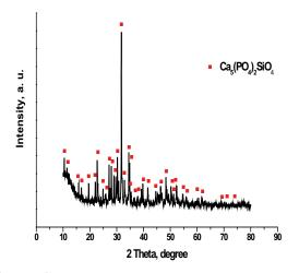
Figure 2. XRD of the prepared G/S hybrid (25:75 wt.%) sample
