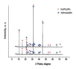
Figure 6. XRD obtained for G/S hybrid materials with 25:75 wt.% (a) and 75:25 wt.% (b) after immersion in 1.5 SBF for 3 days
