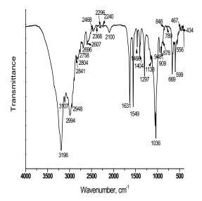
Figure 10. FTIR of the G/S 25:75 wt.% after immersion in SBF for 3 days
