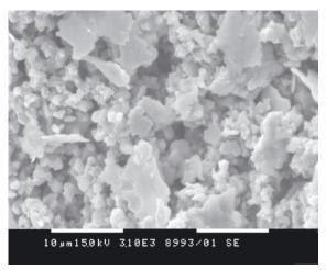
Figure 12. SEM of the G/S (25:75 wt.%) hybrid before immersion in 1.5 SRF
