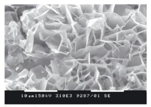
Figure 13. SEM of the G/S (75:25 wt.%) hybrid after immersion in 1.5 SBF
