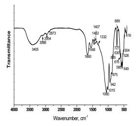
Figure 5. FTIR of G/S hybrid (25:75 wt.%) before immersion in 1.5 SBF
