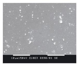
Figure 11. SEM of the G/S (75:25wt.%) hybrid before immersion in 1.5 SBF
