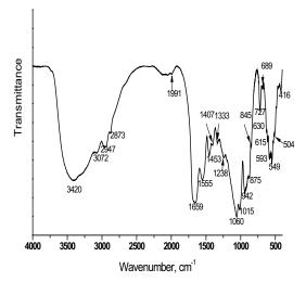
Figure 4. FTIR of G/S hybrid (75:25 wt.%) before immersion in 1.5 SBF
