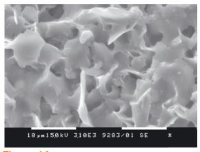
Figure 14. SEM of the G/S (25:75 wt.%) hybrid after immersion in 1.5 SBF
