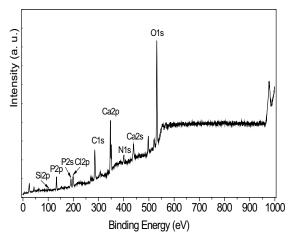
Figure 7. XPS spectrum for obtained G/S hybrid material 25:75 wt.% after immersion in 1.5 SBF for 3 days
