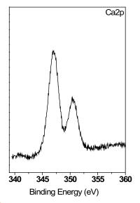
Figure 8. XPS Ca2p spectrum for G/S hybrid material 25:75 wt.% after immersion in 1.5 SBF for 3 days
