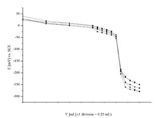
Figure 2. Five titration curves for 2 mL of stearic acid solution (●0.09 M), by a standard TBAH solution of 0.1 M, using pyrite as an indicator electrode in iso-propanol.
