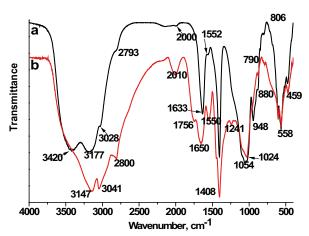
Figure 4. FTIR spectra of collagen/silicocarnotite coatings, before immersion in 1.5SBF with different quantity of collagen and silicocarnotite: 25:75 wt% (a) and 75:25 wt% (b)
