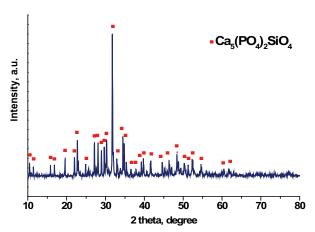
Figure 1. XRD patterns for silica containing sample, thermal treated at 1200°C / 2 h
