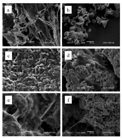
Figure 8. SEM images for pure collagen (a), silicocarnotite (b), silicocarnotite/collagen 75:25 wt% (c), silicocarnotite/collagen 25:75 wt% before SBF (d), silicocarnotite /collagen 75:25 wt% (e), silicocarnotite /collagen 25:75 wt% after immersion in SBF for 3 days (f)
