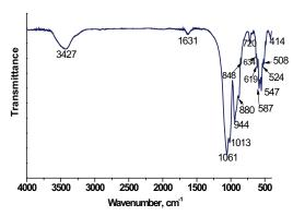
Figure 2. FTIR spectrum of silicocarnotite, heat treated at 1200°C/2 h
