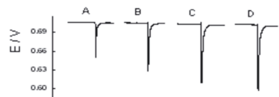
Figure 4. The profiles of adding samples close to the point of bifurcation. Conditions: A=27.0°C; B=28.4°C; C=30.6°C; D=33.5°C. Common Conditions: [MnSO 4 ]=1.13×10 -5 mol L -1 , [KBrO 3 ]=1.75×10 -2 mol L -1 , [Tartrate]=1.05×10 -2 mol L -1 , [H 2 SO 4 ]=0.14 mol L -1 , [Acetone]=8.00×10 -2 mol L -1 , [ p -nitroaniline]=4.50×10 -4 mol L -1
