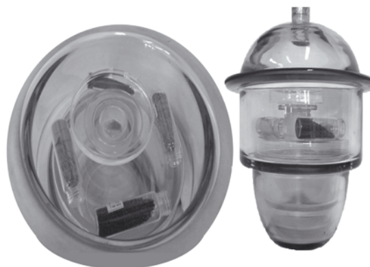
Figure 1. Modified desiccator for soil contamination by vapor treatment method: Petri dish with aqueous solution of PCE, glass vials filled with soil and desiccator cover.
