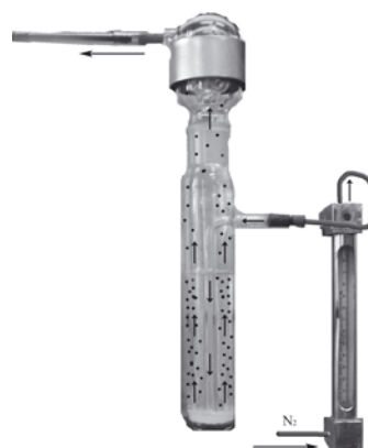
Figure 3. Purge-and-trap laboratory equipment: nitrogen flow meter and controller, stripping column, drops separator and trap with sorption tube.
