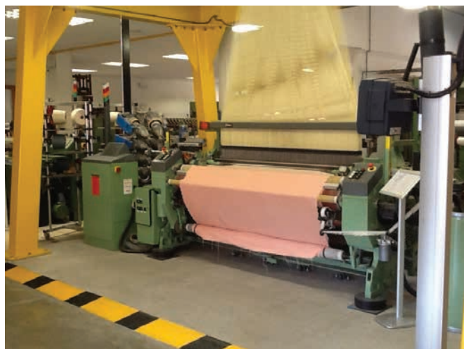
Figure 1. Jacquard loom used to weave the fabrics.
