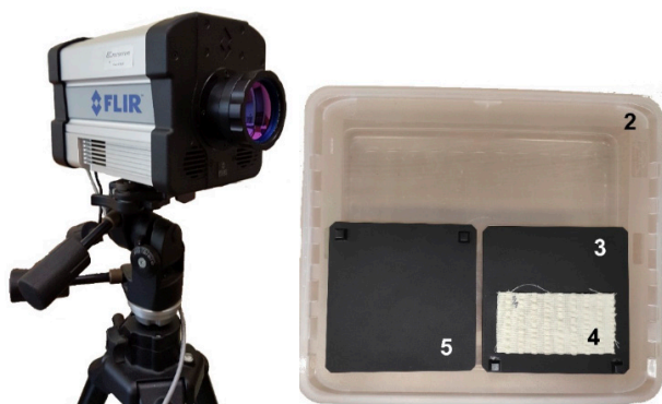
Figure 2. The measuring setup applied in the experiment and its components: (1) FLIR SC6000HS infrared camera, (2) water tank, (3) lower plate, (4) fabric sample, and (5) upper plate.
