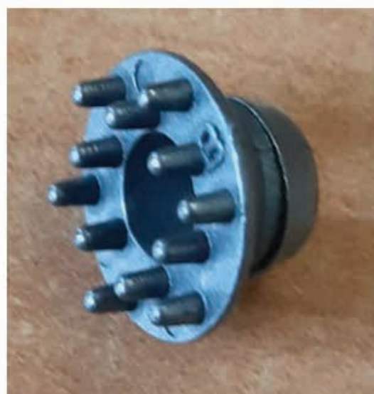
Figure 3. Standard EEG electrodes; gold cup wet electrode (left); and pin-shaped dry Ag/AgCl electrode (right).
