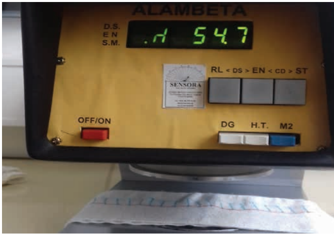
Figure 4. Alambeta testing device for thermal comfort properties [30]
