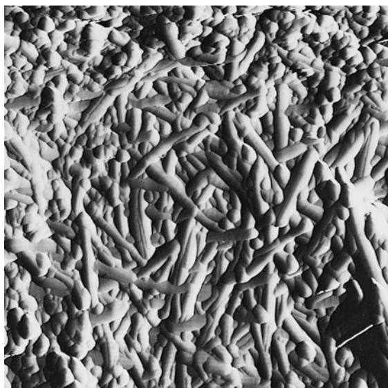
FIGURE 6. HAP reacted with 500 mg/L [Pb_{aq}] . TMAFM image showing botryoidal masses (see top portion of image) and small intergrown needles (scan area = 2.00 \mu\text{m} on a side). SEM (results not shown) revealed aggregates of morphologically indistinct material. XRD results (see Fig. 3e) indicate that the sample was HPY. EDS (results not shown) indicate that the material imaged with SEM was dominated by Pb and P.
