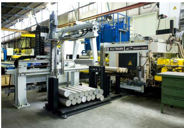
Fig. 3. Magnetic billet heater operating at WeserAlu, Minden, Germany (Courtesy of Zenenergy Power).
