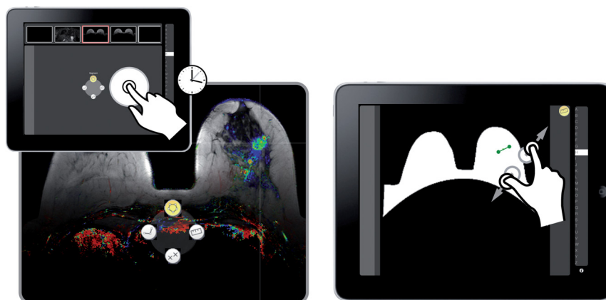
Figure 4: Tap and hold shows a radial menu around the finger on the touch display and on the primary screen (Lepinski et al. 2010). All options that apply to this location, e.g. measurement, are displayed. Measuring the size of a lesion is executed by moving two fingers away from or towards each other.
