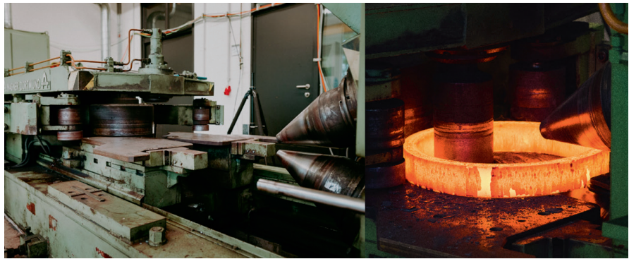
Figure 1. The radial-axial ring rolling machine at the Chair for Production Systems, Ruhr-University Bochum, Germany
