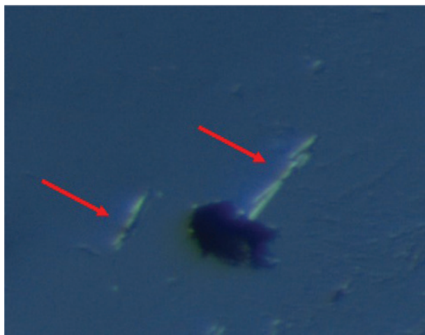
Fig. 1: Needle-shaped crystals of K_5Sn_2OF_{11} (indicated by red arrows) viewed through a polarization microscope.
