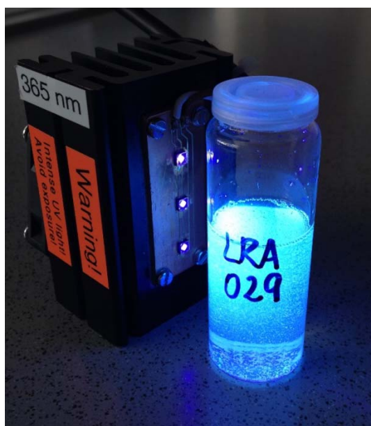
Figure S3: Blue luminescence of \text{EuBr}_2 dissolved in \text{BmimBF}_4 irradiated with UV light (365 nm) after cooling down from 60 °C to room temperature.
