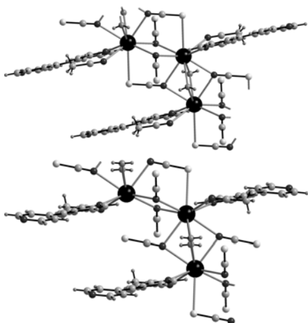
Fig. 10. Part of the chains in the crystal structures of the polymorphs 4I (top) and 4II (bottom). The disorder in 4II is not shown for clarity.
