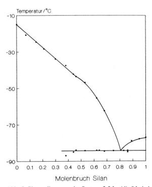
$Abb.\ 5.\ Phasendiagramm\ des\ Systems\ 2.5\text{-}Lutidin/Methyltrichlorsilan}.$
