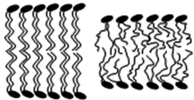
Figure 4: Sketch of the gel (left) below the melting point and the fluid phase (right) of the DMPC LLC. The head groups of the molecules are represented by the black oval.
