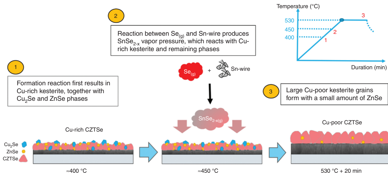
Figure 4: Schematic illustration of the initial growth of Cu-rich kesterite and transition towards Cu-poor kesterite. Added elemental Sn-wire in the graphite box provides \text{SnSe}_{2-x} vapour during the high-temperature dwelling stage of the annealing and leads to Sn incorporation to the absorber.
