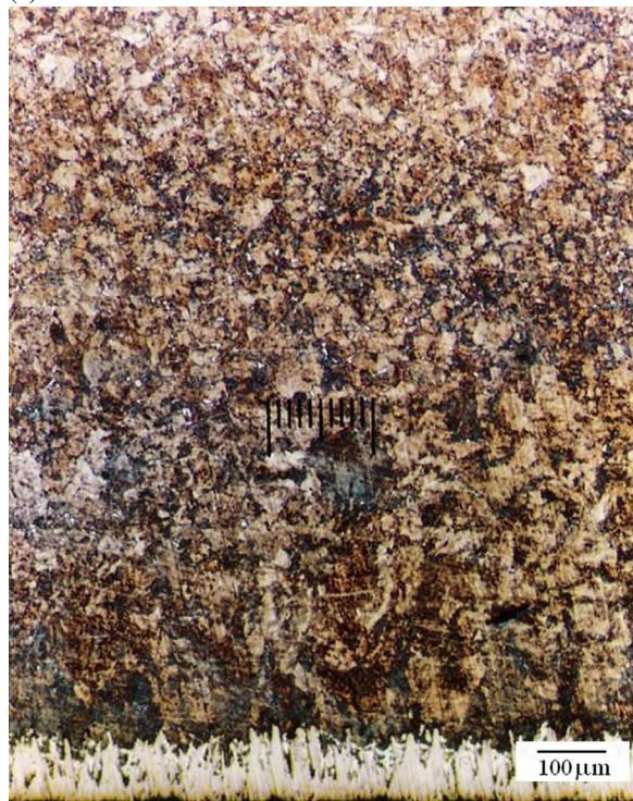
Fig. 1. Optical cross-section of Fe-0.94%Mn binary alloys boronized at 1210 K for 4 h; (a) for alloys of group A; (b) for alloys of group B.
