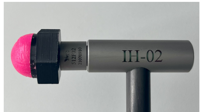
Fig. 1: Impulse hammer Sigmatest IH02 with a custom made silicone tip resembling size and material properties of a small bat.
