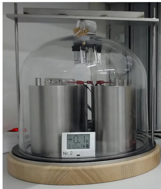
Figure 4: The type-1 glass storage vessel filled with ambient (laboratory-) air at room pressure and molecular sieve 0.4 nm.
