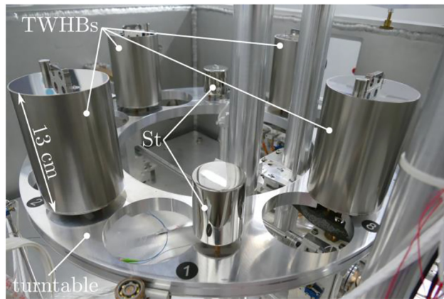
Figure 1: The inner side of the main chamber of the modified Sartorius CCL1007 prototype vacuum mass comparator with the four TWHBs and the four stainless-steel mass standards (St), positioned on the turntable.
