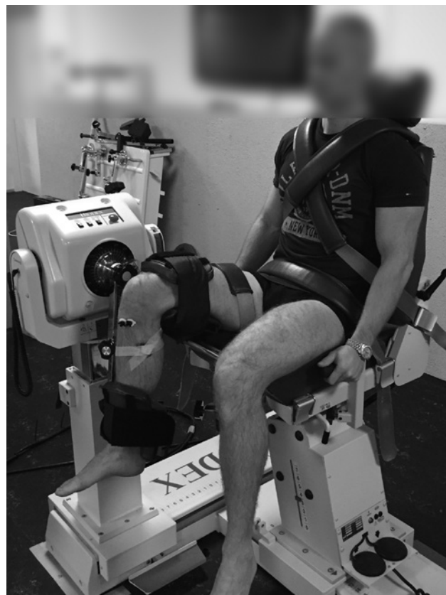
Fig. 1: The picture illustrates the experimental set-up using the isokinetic dynamometer. Here, the participant was comfortably seated with the trunk and lower extremities securely fastened with straps. The lever arm of the biodex passively moved the leg towards extension at a speed of 5^\circ/\text{s} . The participant was instructed to press a button when the stretch sensation in the posterior thigh changed to pain.
