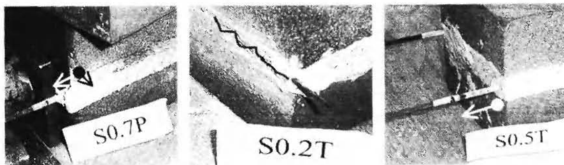
Fig. 2: Different mechanisms of bond failures: de-bond of repointing mortar, splitting on mortar surface, sliding of the strip into the repointing mortar.
