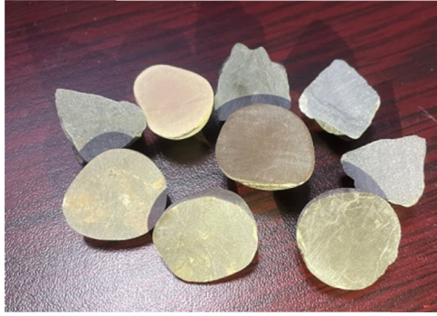
Figure 1: Aggregate with the flat surface cut out.
